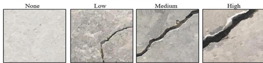
Fig.1 Sample images from Mendeley Concrete Cracking Level dataset
